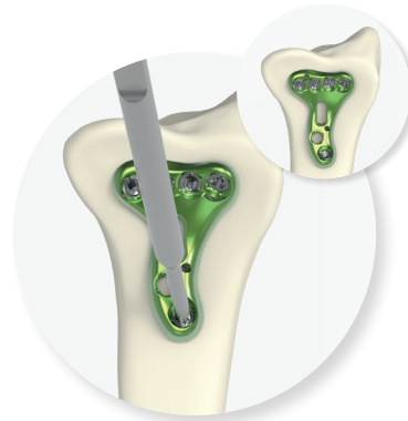
11. Using the T8 screwdriver (ANC910) insert a locking screw (SDT2.4Lxx) into the proximal diaphyseal hole.
